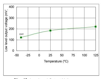
Fig. 43. Low Level Output Voltage vs. Temperature
