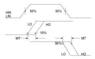
**Figure 5: Delay Matching Waveform Definition**
