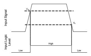
Figure 6: HIN & LIN input thresholds
