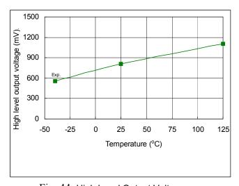
Fig. 44. High Level Output Voltage vs. Temperature
