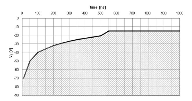
Figure 23: Negative V<sub>S</sub> transient SOA for IRS2607D @ VBS=15V
