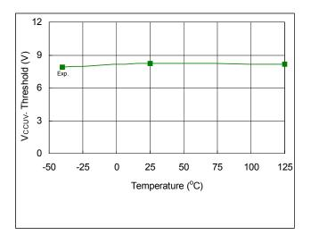
Fig. 41. V<sub>CCUV-</sub> Threshold vs. Temperature
