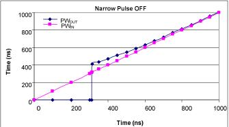
Figure 11: IRS2607D input filter characteristic
