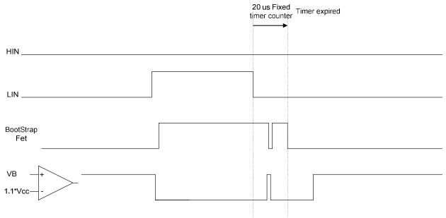
Figure 14: BootFET timing diagram
