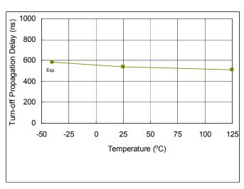
Fig. 30. Turn-off Propagation Delay vs. Temperature
