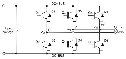
Figure 15: Three phase inverter
