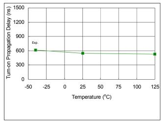
Fig. 29. Turn-on Propagation Delay vs. Temperature
