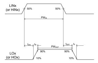
Figure 3: Switching time waveforms
