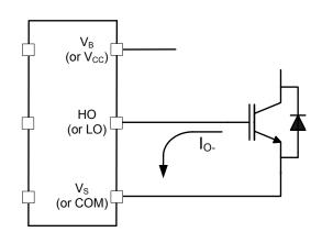
Figure 2: HVIC sinking current
