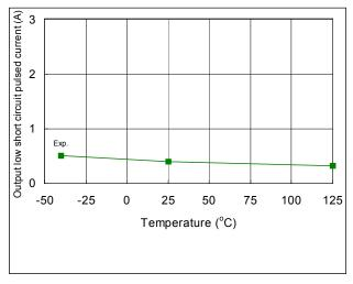
Fig. 34. Output Low Short Circuit Pulsed Current vs. Temperature
