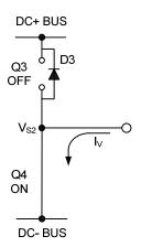
Figure 19: Q4 conducting
