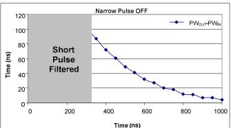
Figure 12: Difference between the input pulse and the output pulse
