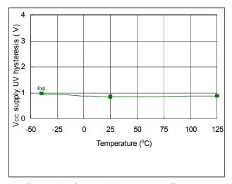
Fig. 36. V<sub>CC</sub> Supply UV Hysteresis vs. Temperature
