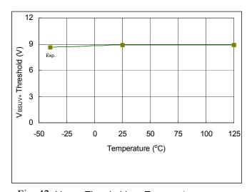
Fig. 42. V<sub>BSUV+</sub> Threshold vs. Temperature
