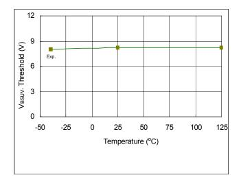
$Fig.~46.~\mbox{V}_{\mbox{\scriptsize BSUV-}}$  Threshold vs. Temperature
