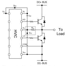
Figure 26: V<sub>s</sub> clamping diode
