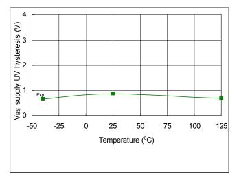
Fig. 37. V<sub>BS</sub> Supply UV Hysteresis vs. Temperature
