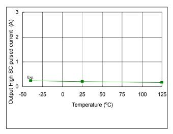
Fig. 33. Output High SC Pulsed Current vs. Temperature
