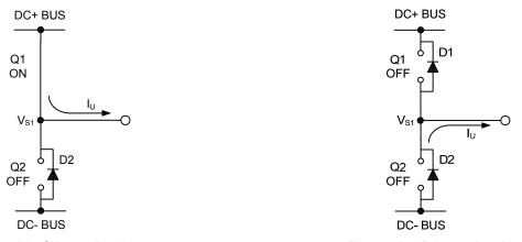
Figure 16: Q1 conducting
