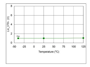
Fig. 48. Lin\_VTH- vs. Temperature
