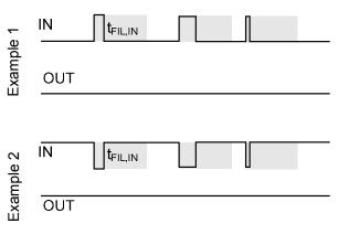
Figure 10: Noise rejecting input filters
