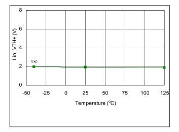
Fig. 47. Lin\_VTH+ vs. Temperature
