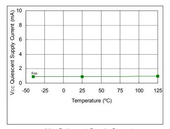
Fig. 38.  $V_{CC}$  Quiescent Supply Current vs. Temperature
