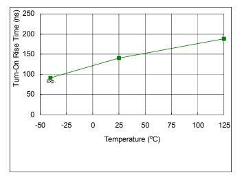
Fig. 31. Turn-on Rise Time vs. Temperature
