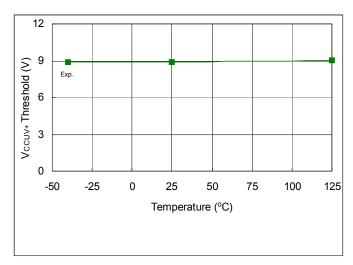
Fig. 40. V<sub>CCUV+</sub> Threshold vs. Temperature
