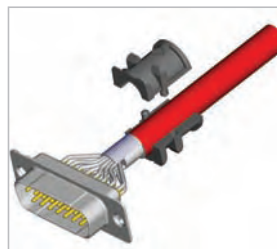
Attach the strain relief around the cable
